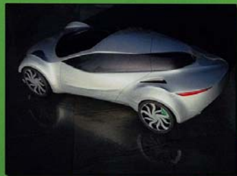
1/4th scale hard model, casted in FRP, polished, painted and taped
